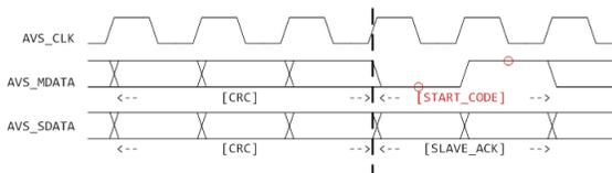
When the master wants to leave idle space between frames, it must complete the last frame of one group (all the way to the rising edge that completes the clock cycle for the last CRC bit), then suspend the clock by driving it low (which allows the slave to cleanly go into idle by sampling a '1' where it would have expected a '0' as part of the '01' start code), and resume the clock when necessary to send the '01'.
